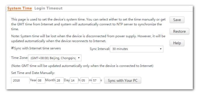
The AP allows you to set the system time by synchronizing the time with the internet or manually setting the time. By default, it is configured to synchronize the system time with the internet.
